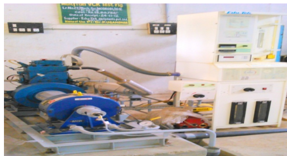
Fig. 3.3: Variable Compression Ratio (VCR) Engine Test Rig
